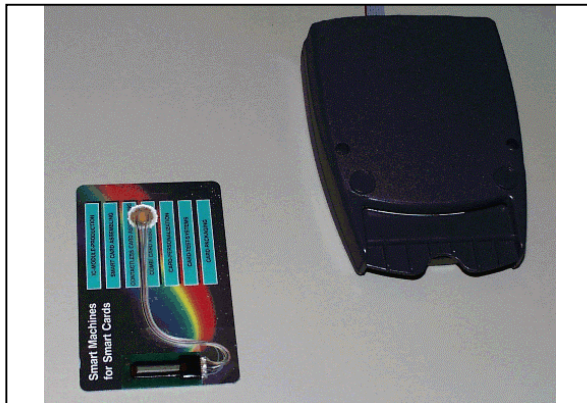
The FingerChip™ is integrated on the smart card, connected to the chip. Here, connected to the smart card connector.
