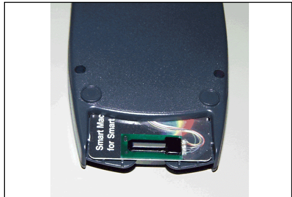
The smart card is inserted in the reader. On this demo, the reader is connected to a PC.
